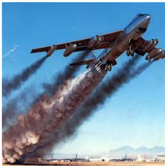
Boeing B-47B rocket-assisted take off on April 15, 1954. (U.S. Air Force photo)
